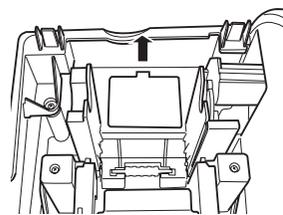
3. Install three new alkaline batteries LR6 ("AA" size) as shown at the right. (Batteries are not supplied with the cash register.) Make sure that positive (+) and negative (-) poles of each battery are properly oriented.
