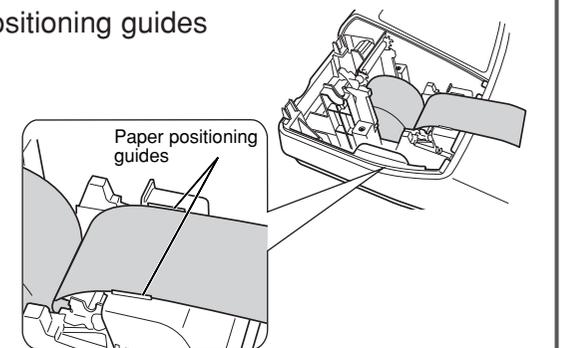
4. While holding down the paper, slowly close the print roller arm, and push down the arm until you hear a click locking the arm. Make sure you securely push down the center of the wing part of the arm as illustrated at the right. The paper will be fed automatically.
