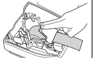
5. Cut off the excess paper using the edge of the inner cover, and replace the printer cover. Press the [↑] key to make sure the paper end comes out of the printer cover and clean paper appears.
