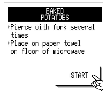
4 Touch START pad. When the sensor detects the vapor emitted from the food, the display will begin counting down the cooking time.
