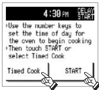
4 Touch number pads 4|3|0 to set the time of day for the oven to begin cooking. Touch START or select Timed Cook .
