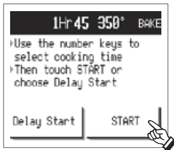
4 Touch number pads 1 4 5 to enter cooking time in hours and minutes. Touch START .
