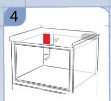
Place electrical outlet in upper back left side in the cavity opening. Can also be installed using an electrical outlet in an adjacent cabinet. Always check electrical codes for requirements.
