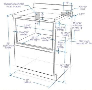
\* Can also be installed using an electrical outlet in an adjacent cabinet within the area where the provided electrical cord can reach. Power cord access hole in cabinet should be a minimum 1 1/2" diameter hole and deburred of all sharp edges.
