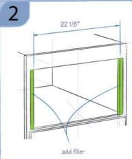
Add vertical fillers to the opening width. The width of the opening should be 22 1/8".
