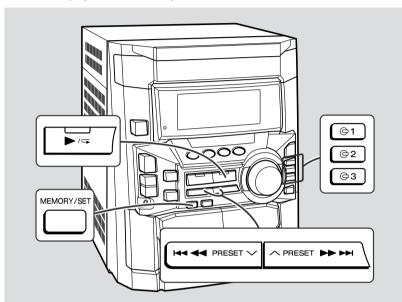
While in the stop mode, press one of the @ 1 - @ 3 buttons to select the desired disc.
