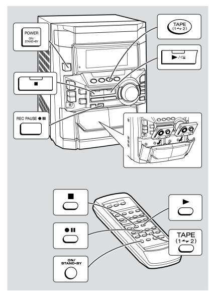
You can record from TAPE 1 to TAPE 2. For recording use only normal tape. Do not use metal and CrO<sub>2</sub> tapes.
