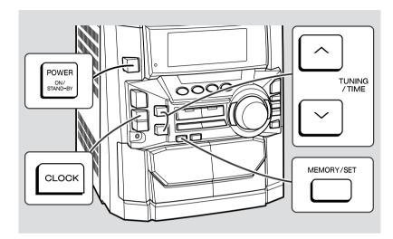
In this example, the clock is set for the 12-hour (AM 12:00) display.
