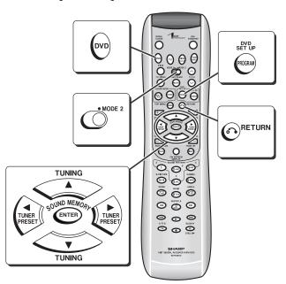
1 Press the DVD button, set the MODE 1/MODE 2 switch to MODE 2 and press the DVD SET UP button.
