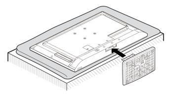
4 Secure the TV stand to your TV with the four provided M4 (10 mm) screws. (These are the short screws.)
