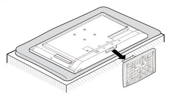
**4** Remove the screws in the mounting holes on the back of your TV, then follow the instructions that came with the wall-mount bracket.
