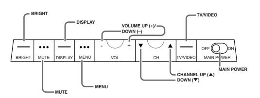
■ The of (MUTE), DISPLAY, MENU, VOLUME UP(+)/DOWN(-), CHANNEL UP(▲)/DOWN(▼), and TV/VIDEO buttons provide the same functions as the buttons on the remote control. (The MENU button has a slightly different function from the remote control button.)
