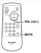
1 Press the VOL (+) to increase sound volume. The segment of indicator increases.
