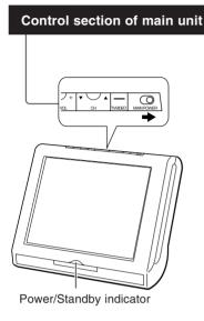
Slide the MAIN POWER switch on the LCD TV set or press POWER on the Remote Control to turn on the LCD TV. The SELECT LAN-GUAGE mode will be displayed.
