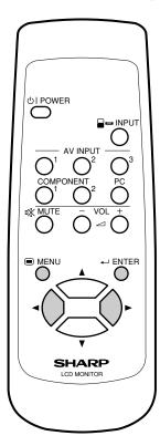
1 Press MENU to display the Menu screen. Press ◆ to move the cursor to SOUND and then press ENTER.
