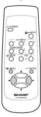
1 Press MENU to display the Menu screen. Press ◆ to move the cursor to OPTION and then press ENTER.
