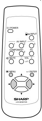
1 Press MENU to display the Menu screen. Press ◆▶ to move the cursor to VIEW and then press ENTER.
