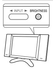
Press **BRIGHTNESS** and adjust the brightness of the display.
