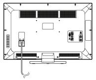
• Place the TV close to the AC outlet, and keep the power plug within reach.
