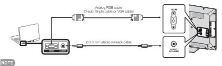
• When using an analog RGB cable, input the audio signal to the AUDIO PC/HDMI terminal of PC IN.
