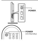
Press **POWER** on the TV or on the remote control unit to turn the power on.
