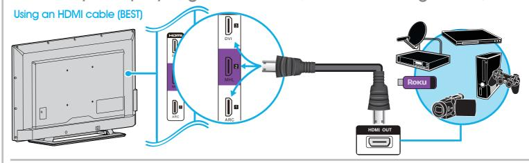
Multi-purpose jack: You can plug any device that uses HDMI into any HDMI jack. However, certain devices must be connected to a DVI, MHL, or ARC jack. See the instructions that came with your DVI, ARC, MHL-enabled device, or Roku Streaming Stick<sup>™</sup> for more information.
