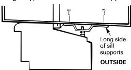
E Adjust the bolt and the nut in each support so that the case is installed with a slight tilt to the outside. Use a level; about 1/2 bubble will be the correct case slant to the outside.
