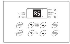
If the display reads "AS", a sensor has failed. Contact your Authorized SHARP Service Center.
