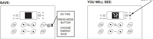
Note: In this mode, the fan will continue to run for 3 minutes after the compressor shuts off. The fan then cycles on for 2 minutes at 10 minute intervals until the room temperature is above the set temperature, at which time the compressor turns back on and cooling starts.
