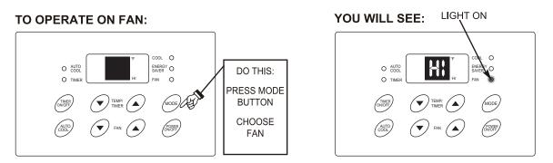
Note: Use this function only when cooling is not desired, such as for room air circulation. You can choose any fan speed you prefer.
