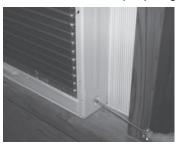
**C** Install control panel back to the front panel.
