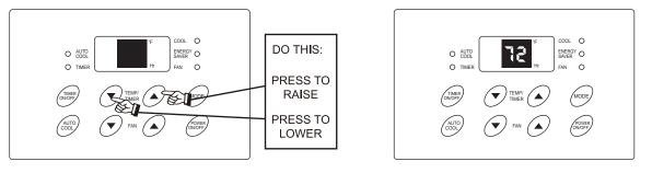
Note: Tap or hold either up(  $\blacktriangle$  ) or down(  $\checkmark$  ) button until the desired temperature is seen on the display. This temperature will be automatically maintained anywhere between 60°F (16°C) and 90°F (32°C). If you want the display to read the actual room temperature See "To Operate on Fan" section .
